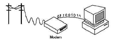
• **Modem** (from **MO**dulator-**DEM**odulator) is a device that modulates an analog carrier signal to encode digital information, and also demodulates such a carrier signal to decode the transmitted information.
