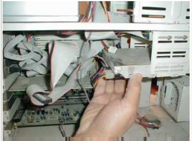
Removing Hard Drive
