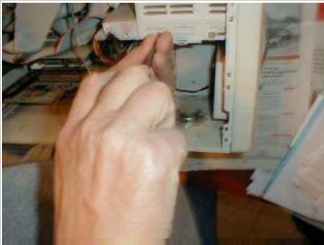
Removing Hard Drive Mounting Screws
