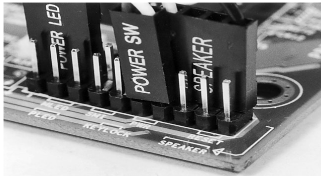
Figure 9: Thin-wire connectors connect the front of the PC case to the mainboard
