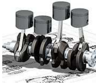
Figure 2.2: An oblique view of a four-cylinder inline crankshaft with pistons.
