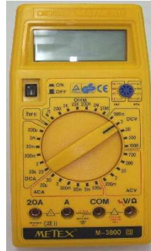
(b) Digital multimeter
